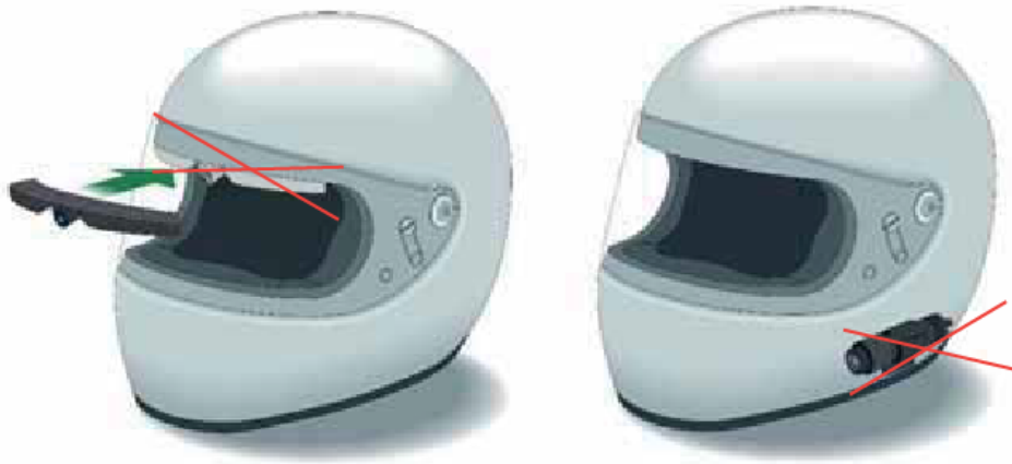
Fig.1 – NOT approved helmet camera installation
